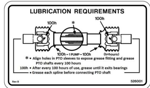
**INPUT & DECK SHAFTS – 100h / Monthly (7 / Shaft - 4 Shafts)**
